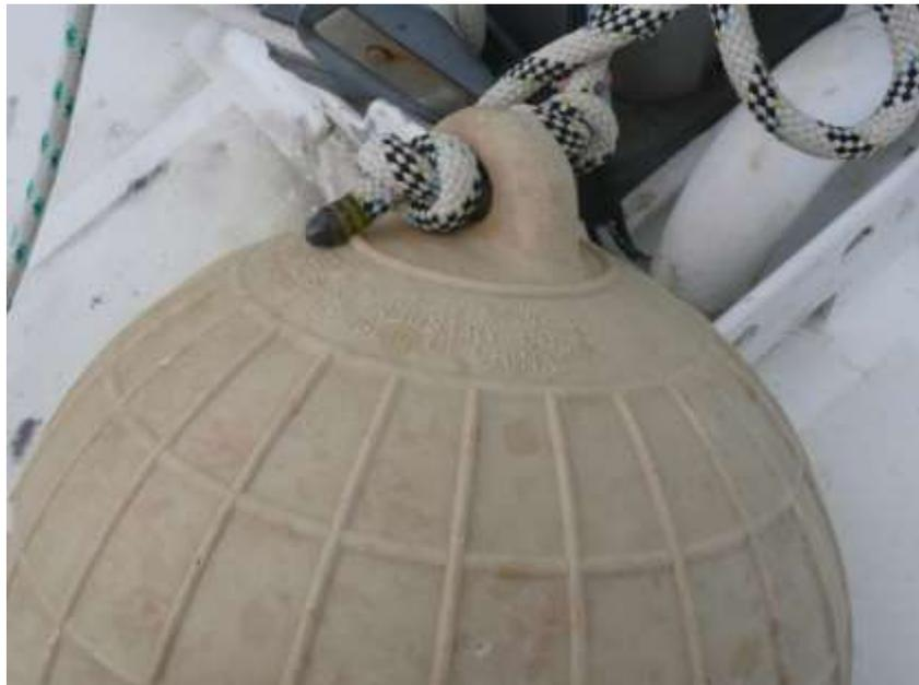
*« Pearl farm » buoys which can be found on any windward beach in the Tuamotus. Snapped on the anchoring chain, they help reducing the wrapping of the chain around coral heads.*
